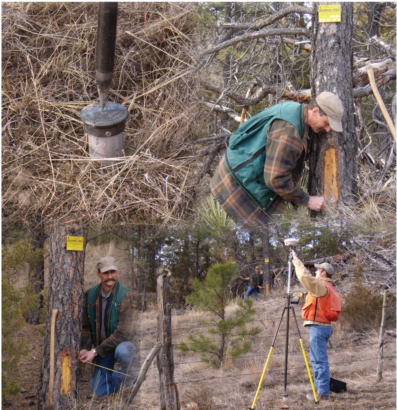
Figure 4-10. A monumented corner, marking and measuring a bearing tree.
